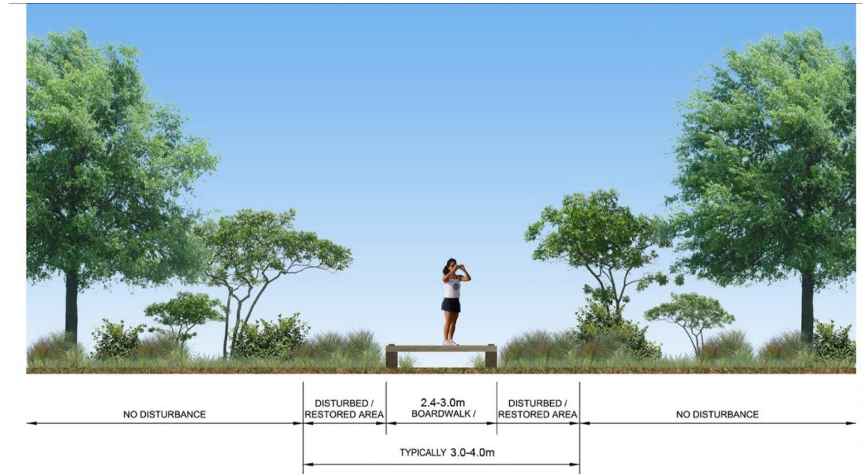
Figure 32: Typical Boardwalk Cross Section
