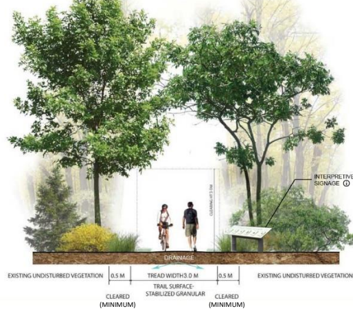
Figure 34: Typical Granular Nature Trail Cross Section
