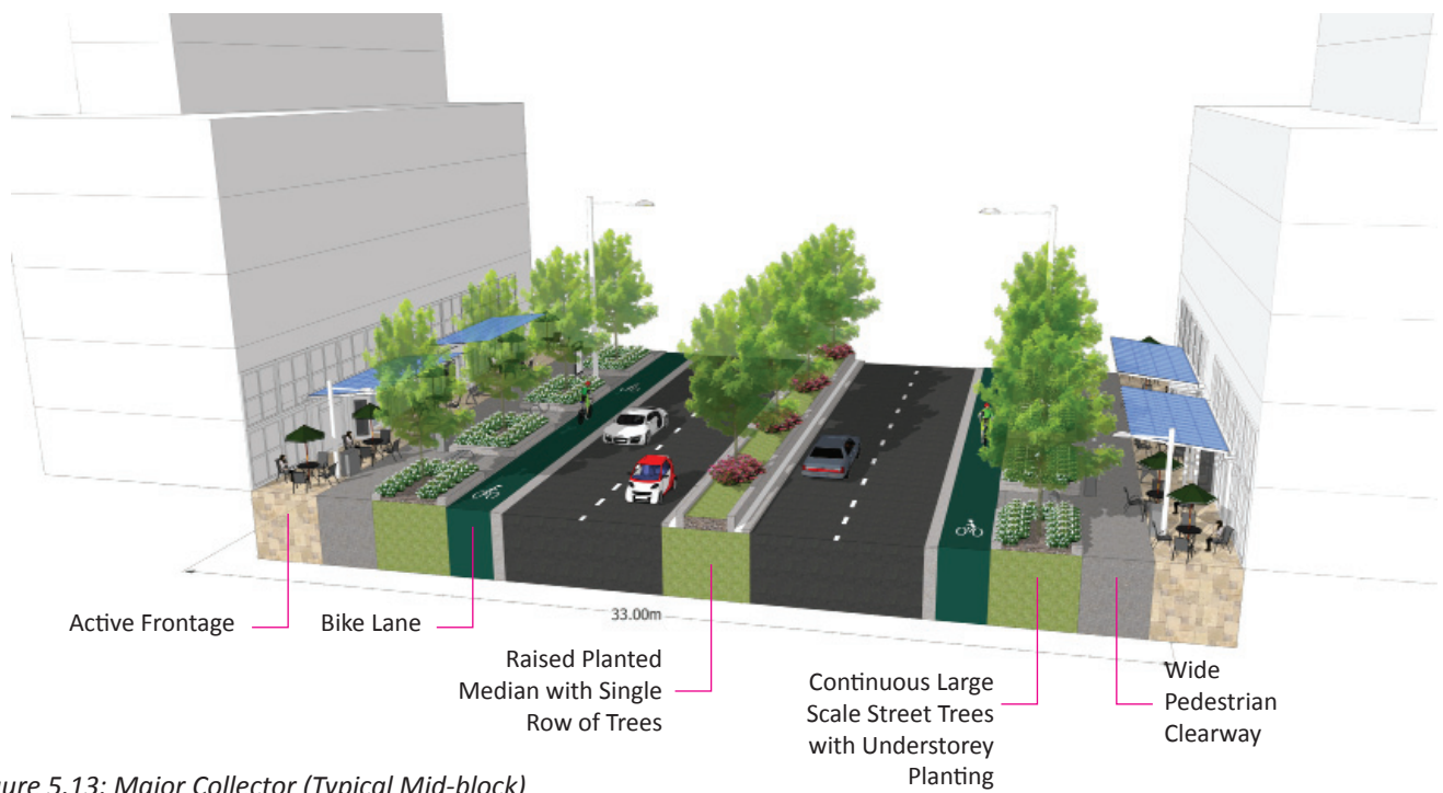
Figure 5.13: Major Collector (Typical Mid-block)
