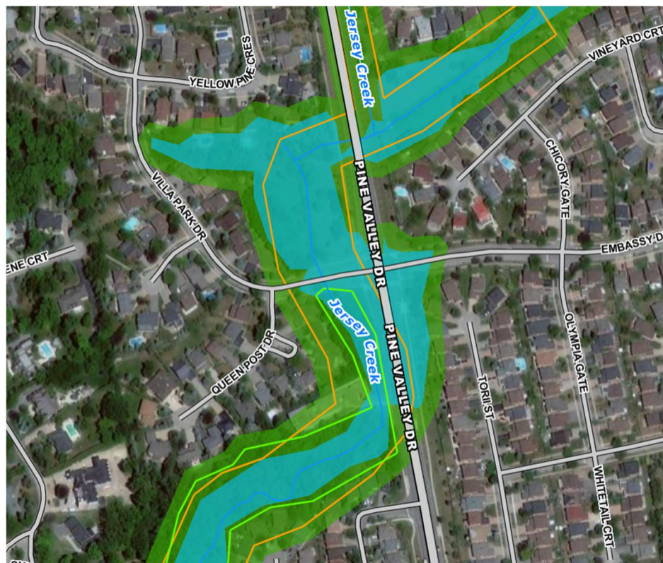
Figure 3.4: Flooding and Regulation Limits (Source: TRCA’s Online Regulation Mapping Tool. Accessed March 10, 2022)
